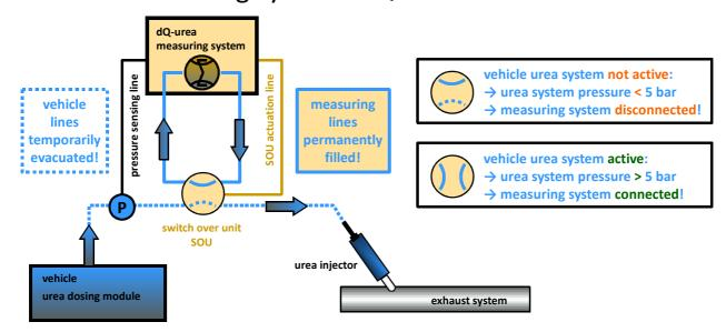
The measuring system dQ-urea is a device which supports an immediate connection to the urea dosing system of the vehicle. The implemented dQ-ad sensor is a directly measuring positive displacement meter working according to the  $\Delta p=0$  – measuring-principle.
