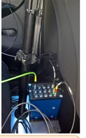
Data acquisition from ADMA via ethernet or CAN interface. A unique test data file with synchronous data of both hunter and target vehicles, plus relative speed and distance.
